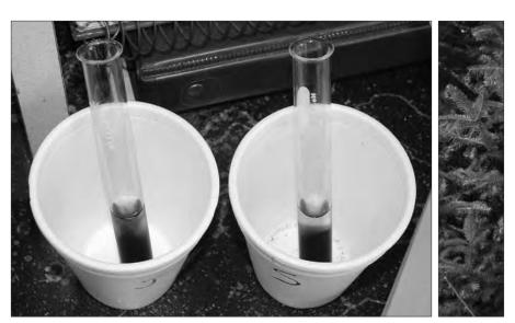
An iodine indicator solution is used to compare the amount of ascorbic acid in various juices and conifer teas.
